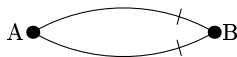
Figure 13. The gadget for equations of the form x + y = 1 . There is a Hamiltonian path from A to B only if one of the ticked edges is traversed.
