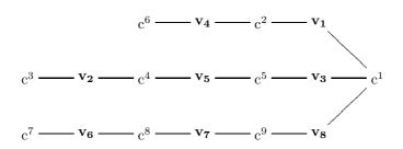
Here variable-nodes corresponding to row j are denoted by  $v_j$ , and clause-nodes corresponding to row i by  $c^i$ . This subgraph has the special property that it is a spanning tree, where the variable-nodes all have degree 2. From these properties by Corollary 4.26 in the next subsection it follows that F is matching lean.<sup>18)</sup>
