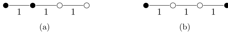
Figure 1: The cut values of the first partition (a) and the second partition (b) are respectively 8 and 6. It follows that single geometric cuts are not always sufficient to generate minimum bisections on the real line.
