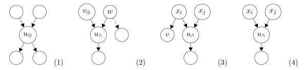
Figure 2: Cases for eliminating gates in  $B_2$ -circuits
