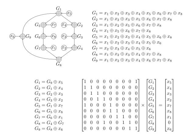
Figure 2: A simple example of a cyclic xor-circuit. In this case all the gates are labeled with  $\oplus$ . The affine functions computed by the gates are shown to the right of the circuit. The bottom row shows the program computed by the circuit as well as the corresponding linear system.
