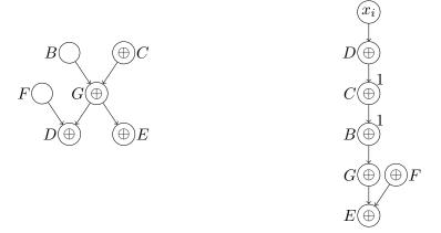
Case 1: under G=0, the gate G is removed, B is replaced by C, D and E are replaced by their other predecessors.
