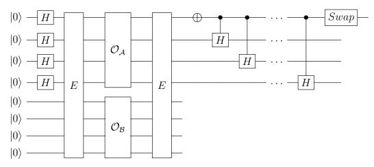
Figure 6: Circuit describing one component of the quantum protocol. The output of this component is the outcome of the Swap test. The final circuit is obtained by taking a threshold of the outputs of  $O(\log^2 N)$  copies of this circuit.
