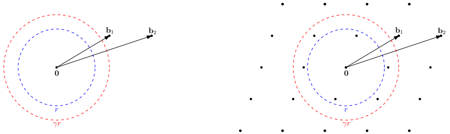
Figure 2: Left: An instance of \gamma -GapSVP consisting of a basis \mathbf{B} = (\mathbf{b}_1, \mathbf{b}_2) and r > 0 . The goal is to decide whether there exists a non-zero lattice vector of norm at most r (i.e., there exists such a vector inside the blue circle), or if all non-zero lattice vectors are of norm greater than \gamma r (i.e., all such vectors are strictly outside the red circle) when one of these cases is promised to hold. Right: Looking at lattice points in \mathcal{L}(\mathbf{B}) near the origin shows that the instance is a YES instance of \gamma -GapSVP because the non-zero lattice vectors \pm(\mathbf{b}_2 - \mathbf{b}_1) are inside the blue circle of radius r .
