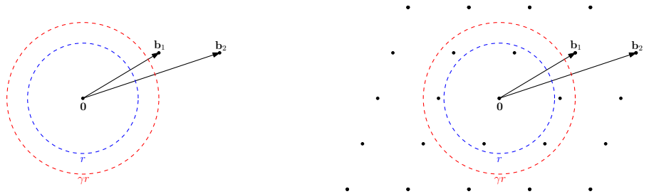
Figure 2: Left: An instance of \gamma -GapSVP consisting of a basis \mathbf{B} = (\mathbf{b}_1, \mathbf{b}_2) and r > 0 . The goal is to decide whether there exists a non-zero lattice vector of norm at most r (i.e., there exists such a vector inside the blue circle), or if all non-zero lattice vectors are of norm greater than \gamma r (i.e., all such vectors are strictly outside the red circle) when one of these cases is promised to hold. Right: Looking at lattice points in \mathcal{L}(\mathbf{B}) near the origin shows that the instance is a YES instance of \gamma -GapSVP because the non-zero lattice vectors \pm(2\mathbf{b}_1 - \mathbf{b}_2) are inside the blue circle of radius r .
